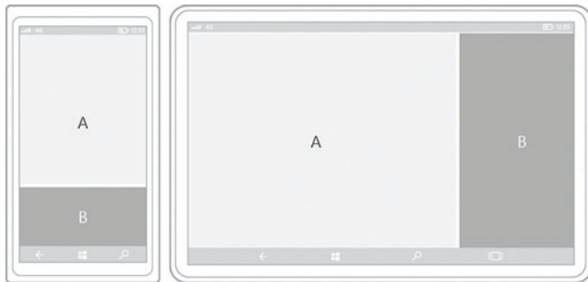
Figure 2 Reposition Frames to Take Advantage of Larger Screens
